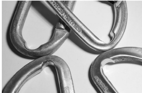
[Above] Deeply grooved carabiners. Replace any carabiners that look like this. Black Diamond
